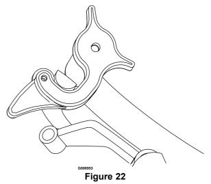
2. Adjust the linkage length by loosening the jam nuts at both ends of the linkage and rotating the linkage in the ball joints. Lengthen the linkage if the tire is turning in reverse and
